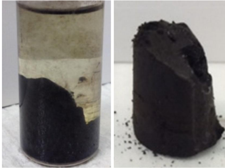
Figure 5.5 Pictures of a wet gel (left) and an aerogel (right) prepared via the oxidation-induced route (MUA + H 2 O 2 ). The monolith (right) has a density of \sim 0.027 \text{ g/cm}^3
